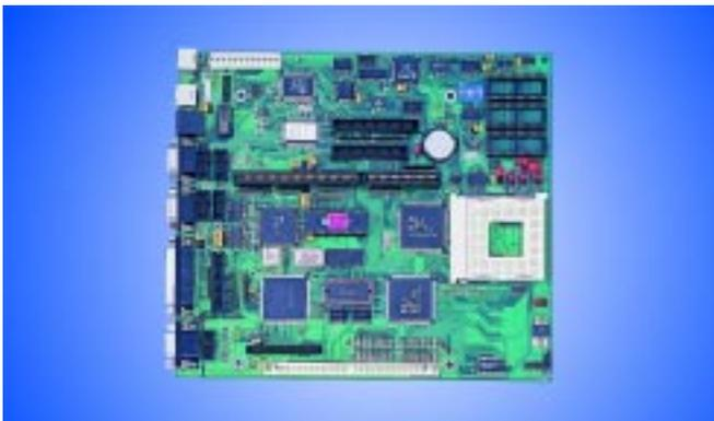
*POS-460 Rev.B1 486-based POS Control Board*
