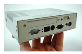
Advantech's MBPC-200 3.5" Biscuit PC chassis line has added the new PCM-5822 half-size Biscuit SBC as one of its board options. The PCM-5822 brings with it a powerful TV-out function as well as a new switching power regulator and low-power GXmLV-200/2.2 V processor. For ease of use and convenience, all cables connect directly to the front panel. AV as well as S-Video connectors are also both provided on the front panel to accomodate all your
