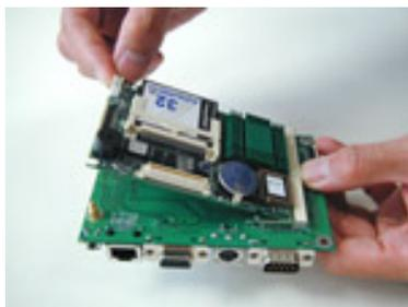
The much anticipated CPC-2420 is now available. This new tiny carrier board comes with a SODIMM socket for carrying the CPC-2245/N Mini Biscuit SBC and has standard I/O connectors such as VGA, LCD, LAN, FDD, IDE, serial ports and a printer port.
