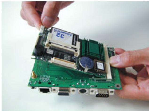
Inserting the CPC-2245/N into the CPC-2420 Carrier Board
