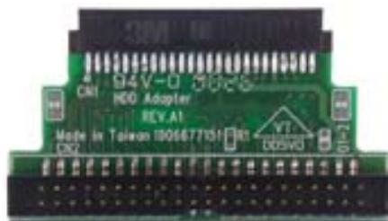
CompactFlash to HDD Adapter
