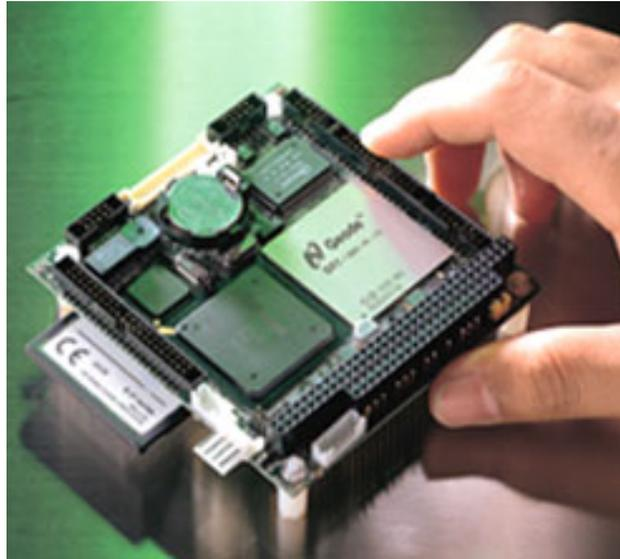
The PCM-3350 is of course great for rugged industrial applications typically associated with PC/104 boards, but with such a powerful processor/system chipset, it is also great for applications such as medical equipment, small Internet appliances and other embedded controllers. Think of the PCM-3350 as a super small desktop computer, ready to go where you need it.
