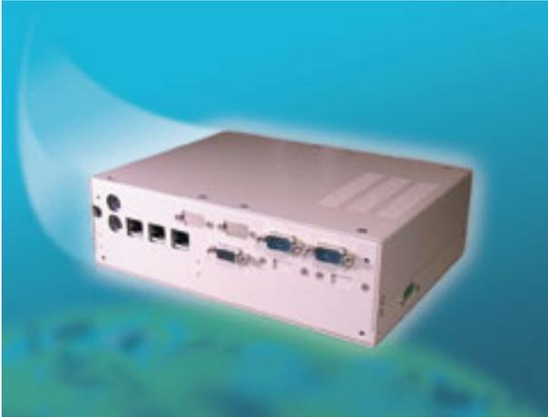
A new family member has just joined the [MBPC-300](#) MicroBox PC series. The new member, MBPC-300-9576F, is a MicroBox 5.25" Biscuit PC Chassis, which supports the PCM-9576F single board computer. The PCM-9576F is a socket 370 Pentium® III SBC that supports Pentium® III /Celeron™ processors up to 850 MHz. The PCM-9576F features three-LAN capability, which makes it flexible and scalable for network administration. The PCM-9576F offers customers the option to choose onboard hardware to
