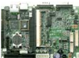
Advantech is proud to announce the PCM-9372, its new 3.5" SBC offering. Adopting the embedded low power VIA Eden processor, this board can operate without a fan at temperatures up to 60° C (140° F) and typically consumes under 12 Watts while
